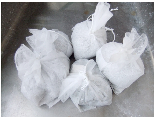
Fig.3 Mesh baggs for immersing paper powder.
